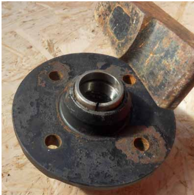
Fig. 40: Put the new shell home
