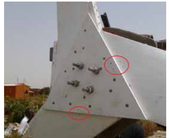
Fig. 18: Marks on blades and triangle
