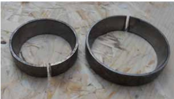
Fig. 39: Cut the shell with an angle grinder
