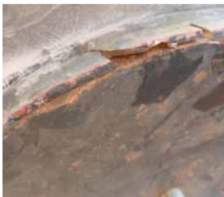
Fig. 33: Cracks in resin in the rotor edge
